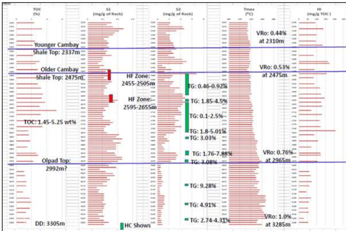
Fig. 7: Geochemical log of Cambay shale section of well WELL-E (Chandra et al., 2017)
