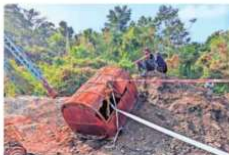
The box used by rescuers to pull out survivors from the rat hole mine at Umrangso in Assam. Express
