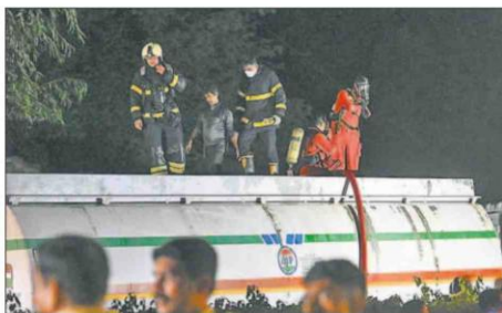
Fire brigade personnel decant benzene from the affected tanker into an empty tanker after the leak was reported. RAJU SHINDE/HT PHOTO
